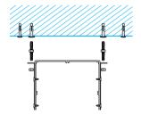
Installing studs on the ceiling and fixing mounting corners on the studs using screws
